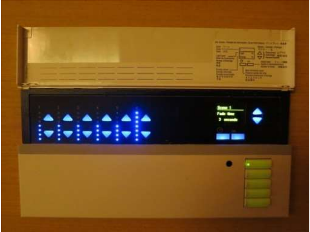
The Keypad offers a user-friendly front-end interface to activate preset scenes.
